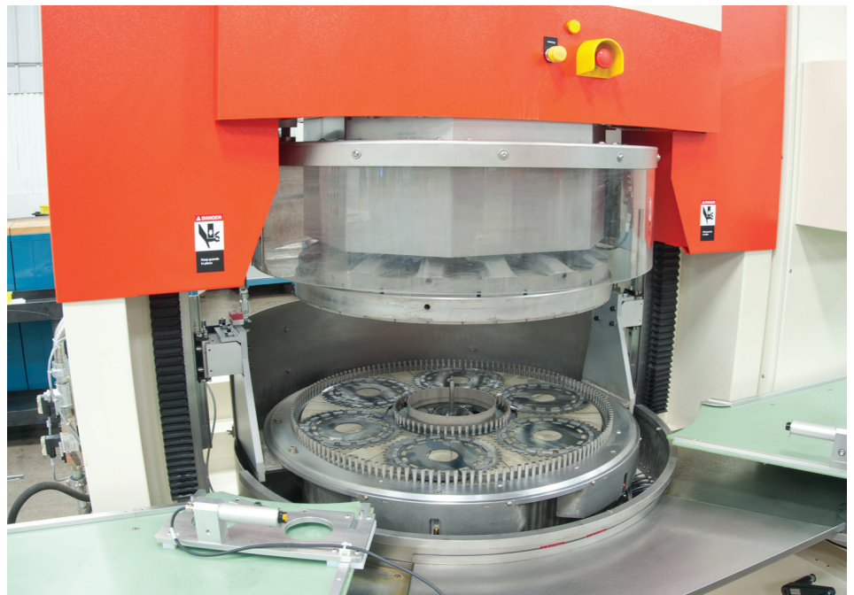
One of two Stahli DLM 705 double-disc grinders Aggressive Grinding Service uses to grind carbide discs with ATI's hybrid metal-bond, induced-porosity wheels.
